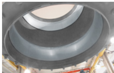
Bellows fitted with inner sleeve to prevent pressure loss from flow resistance and to avoid vibration induced by turbulences
