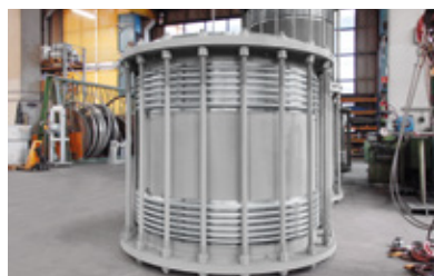
Rounded anchoring elements around the circumference to absorb pressure reaction forces
