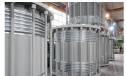
Five of 70 expansion joints following internal visual inspection
