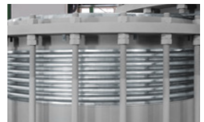
Total of 12 convolutions enable required movement absorption
